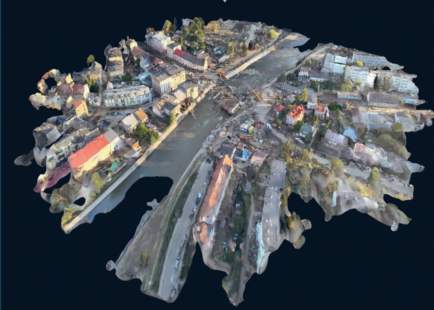
DEADLINE. A measurable 3D model of urbanised infrastructure. Used for initial assessment of road passability for delivery of aid to those in need and forward-looking planning of subsequent rescue and reconstruction activities.
